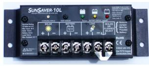
The SS-10L is a very popular solar controller, and sold on many solar oriented web sites and stores. It has a very solid look and feel when held in one's hand. This 10 Amp controller with LVD function, is a sealed "potted" module with mounting brackets and terminal posts, making repair service a bit more difficult. GTIS also has these units at 20
