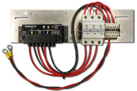
sense terminals. The voltage drop is created by the high enough load currents and the typically small diameter wire that some people use. This might explain the thinking of Morningstar, however their design is a compromise of possible conditions at best. The C-12 Controller allows the savvy technician person to make fine adjustments for each unique installation in the field.
