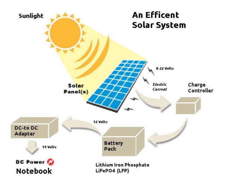
These are the major components of a village system that desires to be **energy efficient**. Note that there is no inverter here, but rather the DC-to-DC auto adapter in the sub-systems that make for a more energy efficient operation. In a cost sensitive situation (local level churches and communities in the third-world) every joule of energy conserved is important per unit cost. Such communities struggle with resources; practical costs are very important.
