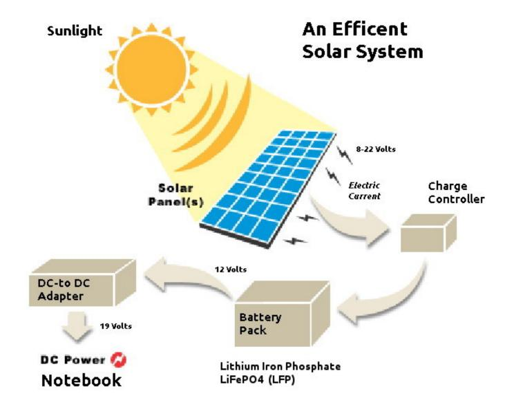
These are the major components of a village system that desires to be **energy efficient**. Note that there is no inverter here, but rather the DC-to-DC auto adapter in the sub-systems that make for a more energy efficient operation. In a cost sensitive situation (local level churches and communities in the third-world) every joule of energy conserved is important per unit cost. Such communities struggle with resources; practical costs are very important.
